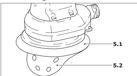
The self-adhesive sanding material (5.2) is simply pressed onto the sanding base (5.1) and held safely in place by the Stickfix sanding base velcro surface.
